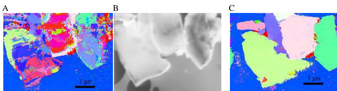
Fig. 7 (a) Orientation mapping of mayenite crystals without precession; (b) Virtual bright field; (c) Orientation map obtained with precession angle of 0.35^\circ
