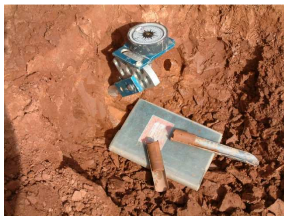
Figure 4 – In situ orientation of drilled cores
