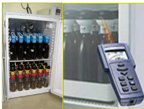
Figure 5. Manometric respirometers used to determine carbon mineralization and indirectly the biodegradation of chemicals in water and soil (Photo from the authors).
