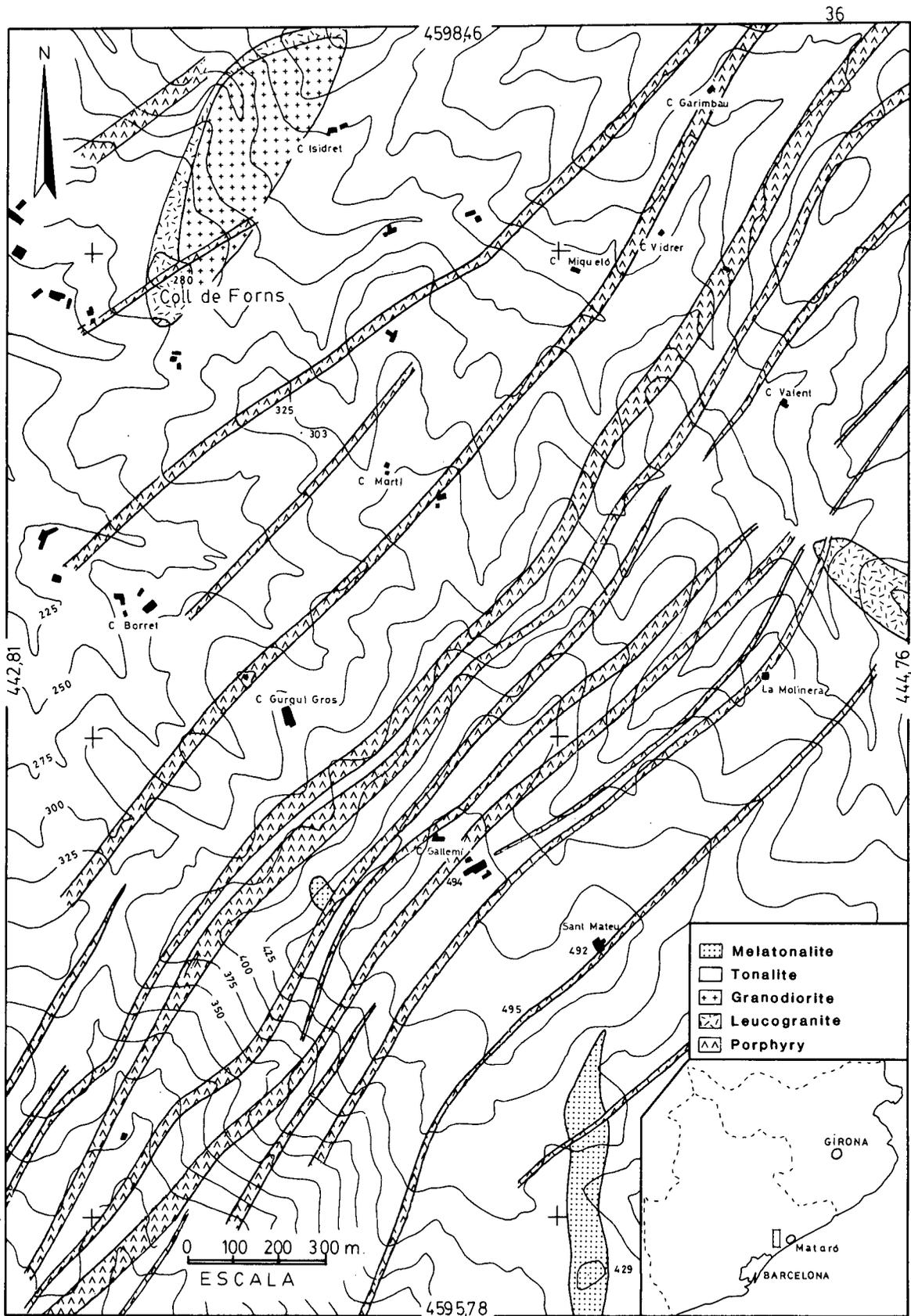
Figure 4.- Detailed map of the dyke swarm of Sant Mateu area (Southern Montnegre) which consists mainly of granite and granodiorite porphyries.
