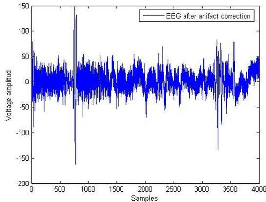
**Fig. 5** EEG signal after subtracting the artifacts detected by the artifact corrector module.
