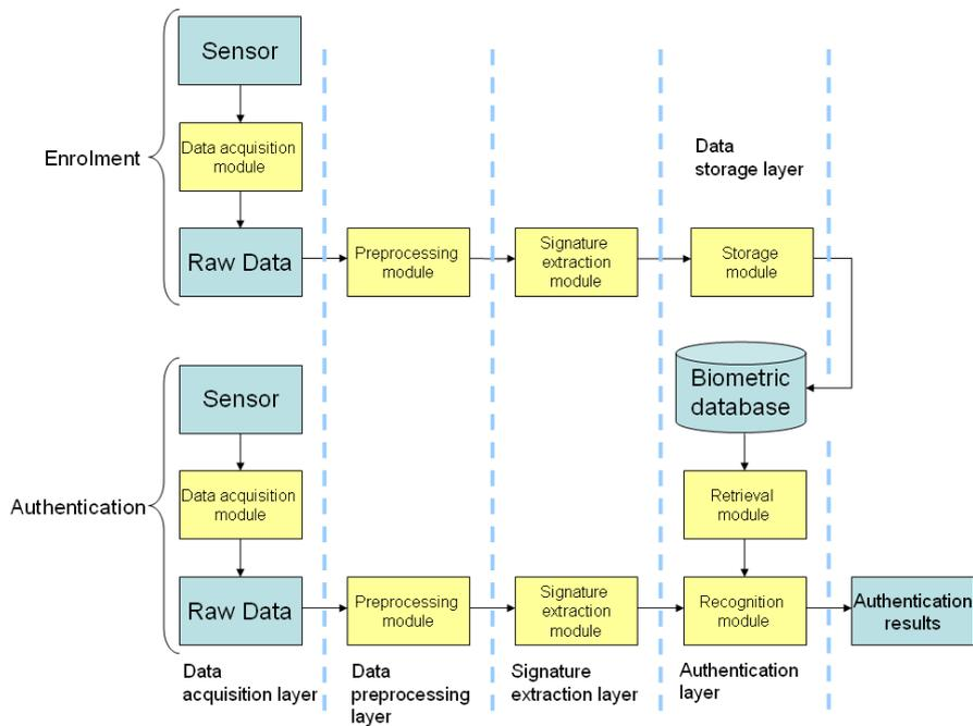
**Fig. 1:** Common architecture of a biometric system.
