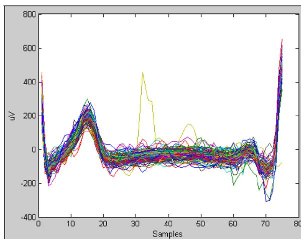
Figure 3.13: ECG waveforms after the resampling (normalisation)
