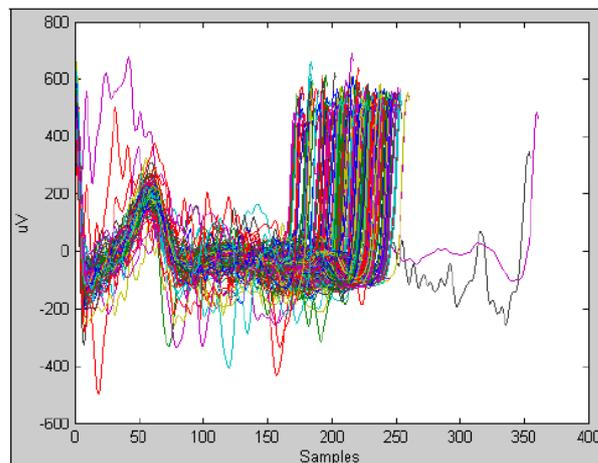
Figure 3.9: ECG waveforms that are considered correct after the first outlier detector
