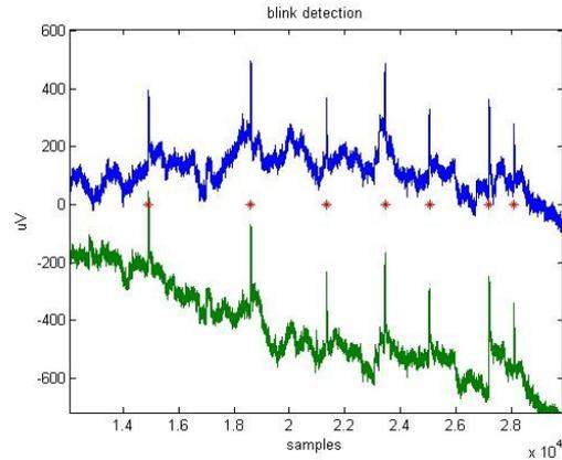
**Fig. 8** EOG sample recorded by ENOBIO. The blue and green lines correspond to FP1 and FP2 respectively. The Red crosses mark the position in the signal where a blink is automatically detected by our algorithm.
