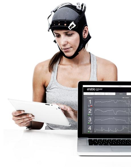
Figure 5.6: Frontal view of the ENOBIO sensor. The data acquisition software can also be seen
