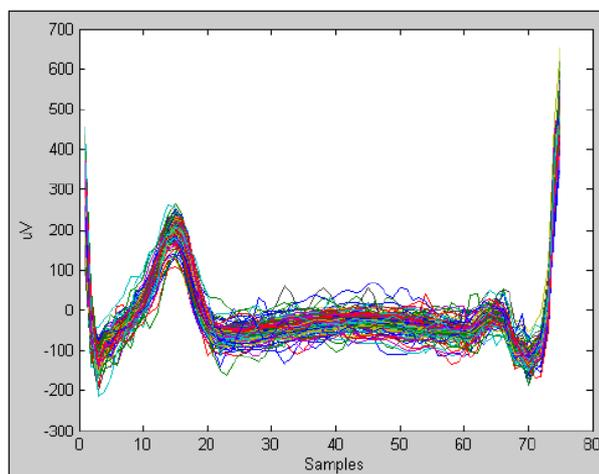
Figure 3.15: ECG waveforms considered correct after the third outlier detector
