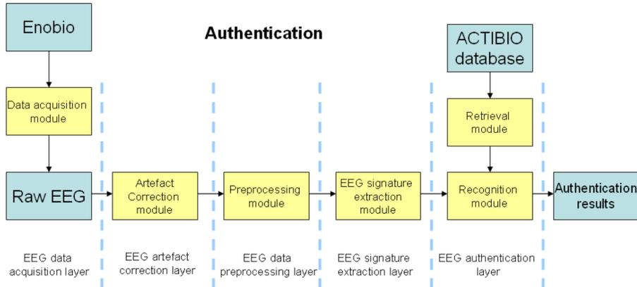
Figure 3.5: Scheme of the EEG authentication process
