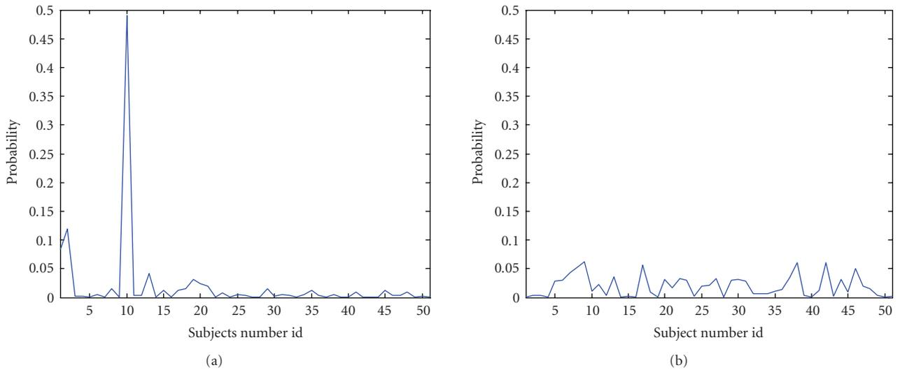
FIGURE 1: PDF for normal situation for subject 10 (a) and for intruder situation (b). In (a), notice that if a probability threshold is set to 0.15, subject 10 will be authenticate only if he claims to be subject 10. In (a), the intruder would not be authenticated in any case.
