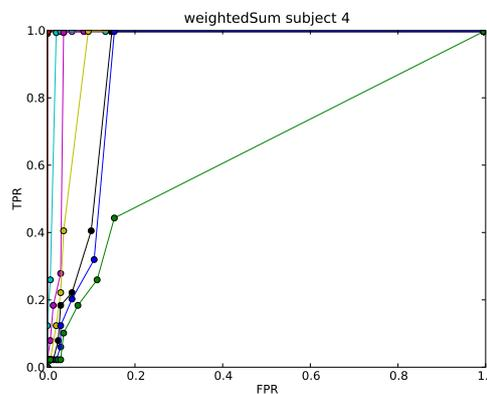
Fig. 7. Example of the extensive search procedure in the parameterization of the weighted sum operator for fusing subject 4 EEG and ECG modalities. Not all parameter results are shown for the sake of clarity. The ROCs (color coded) and its corresponding AUCs are computed on the fusion result. The parameters deliver several ROCs from optimal (red) to worst (green).
