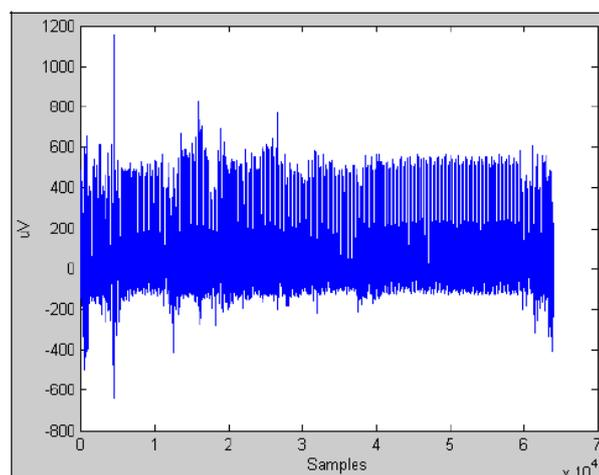
Figure 3.7: Band filtered ECG signal. We can see that the high frequency drift present in fig. 3.6 around sample  $0.5 \times 10^4$  appears now as a strong peak. The ENOBIO sampling rate is 250 Hz
