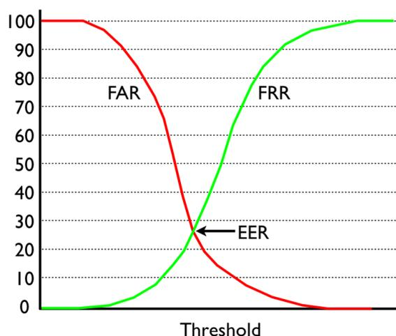
Figure 3.16: FAR-FRR diagram. The EER is given by the crossing of both curves
