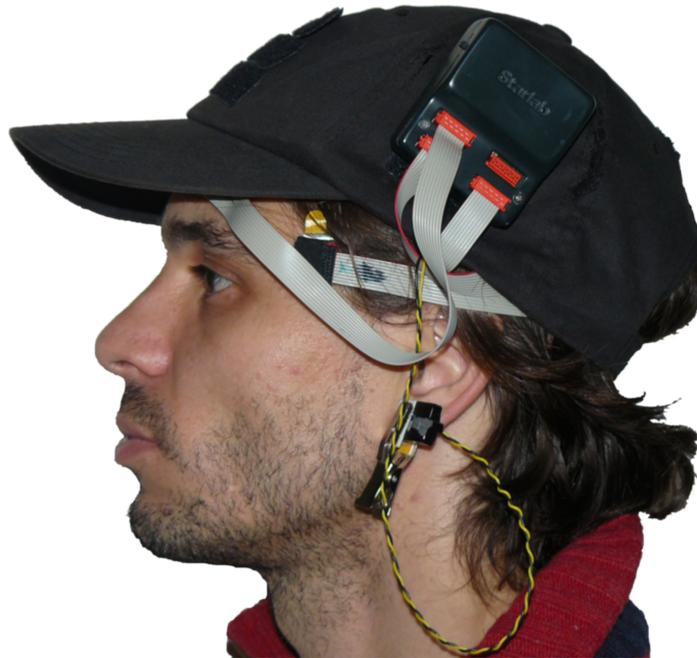
In Figure 1.2, a sample of EEG recorded with ENOBIO is shown. An ECG sample data is also shown in Figure 1.3. Notice that the EEG amplitude is typically about 60 microvolts while ECG amplitude is typically about 1000 microvolts, therefore it is always more complicated to obtain a good EEG recording than an ECG, as the signal to noise ratio is easier to maximize with a stronger signal. No pre-processing has been done on these sample signals.
