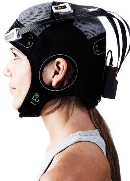
Figure 5.5: Side view of the ENOBIO sensor in its EEG cap configuration
