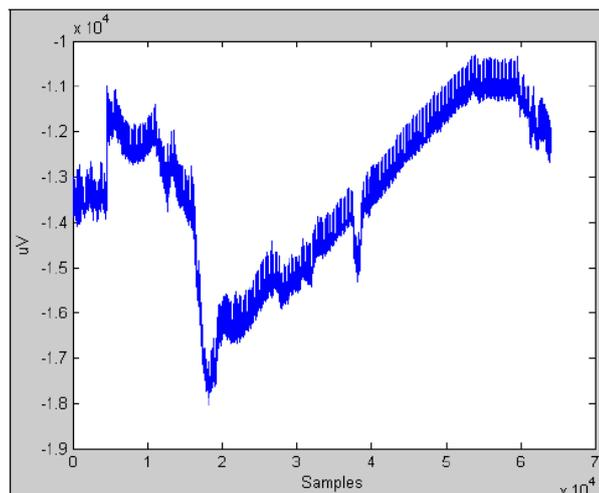
Figure 3.6: Sample of ECG raw data captured with ENOBIO. We can see typical low frequency drifts in the signal. We can also observe a high frequency drift around sample  $0.5 \times 10^4$ . The ENOBIO sampling rate is 250 Hz
