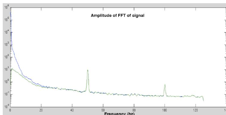
Figure 3.4: Spectrum before (blue) and after (green) applying the artefact corrector
