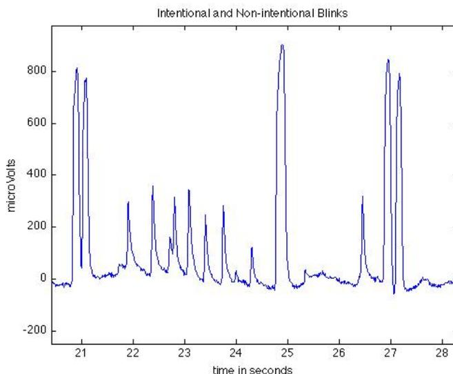
Figure 1.5: Sample of an EOG recording with the ENOBIO sensor. The electrodes were placed above and under the right eye and thus the eye blinks can be observed
