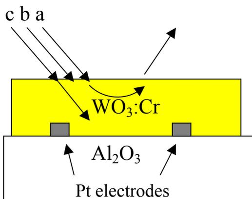
**Fig. 9:** Schema of influence of catalytic activity on sensor response: a) too high catalytic activity, b) low catalytic activity and c) appropriate catalytic activity.
