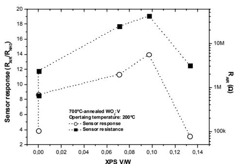
**Fig. 3:** Evolution of sensor resistance and sensor response of 700°C-annealed  $\text{WO}_3:\text{V}$  with XPS V/W ratio.
