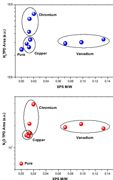
**Fig. 4:** TPD area of  $\text{N}_2$  and  $\text{N}_2\text{O}$  as functions of additive superficial concentration.
