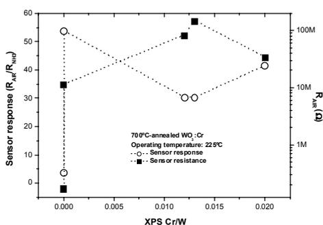
**Fig. 5:** Evolution of sensor resistance and sensor response of  $700^\circ\text{C}$ -annealed  $\text{WO}_3:\text{Cr}$  with XPS Cr/W ratio
