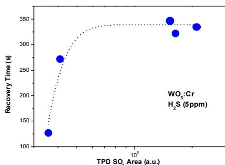
**Fig. 10:** Dependence of recovery time with TPD  $\text{SO}_2$ -area for  $\text{WO}_3\text{:Cr}$ .
