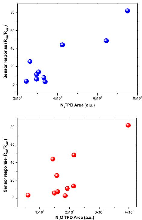
**Fig. 6:** Correlation between sensor response to ammonia (500 ppm at 200°C) and TPD areas of  $\text{N}_2$  and  $\text{N}_2\text{O}$ .
