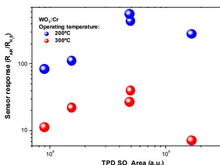
**Fig. 8:** Sensor response of  $\text{WO}_3\text{:Cr}$  as a function of TPD  $\text{SO}_2$ -area.
