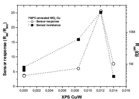
**Fig. 2:** Evolution of sensor resistance and sensor response of 700°C-annealed WO<sub>3</sub>:Cu with XPS Cu/W ratio.
