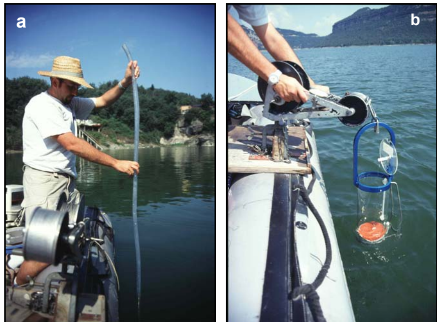
Photo M.1 We collected water samples using two types of sampler: a) Plankton tube sampler. a) Limnological water sampler (UWITEC).
