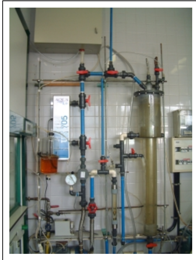
Figure 4.4. Reactor, UV and UVA photoreactor
