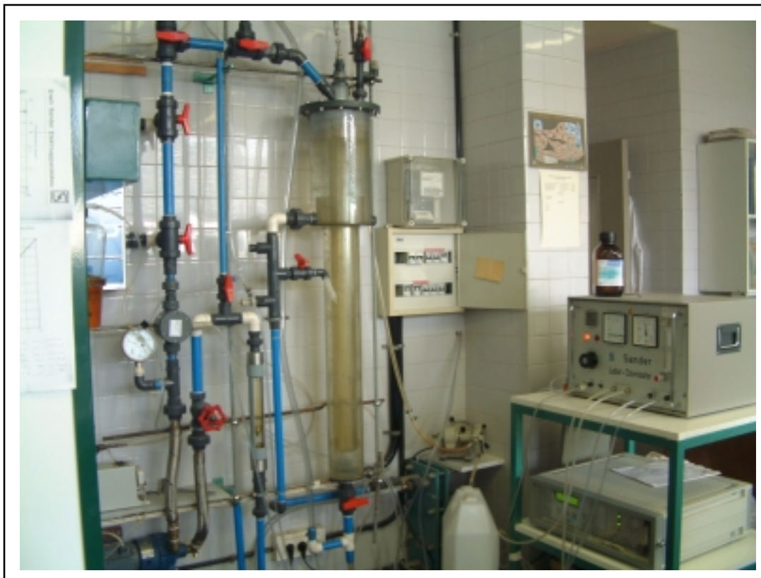
Figure 4.5. Installation, ozonizer and ozone measurer.
