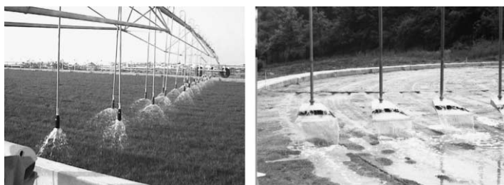
Figure 5 Emitters adopted for secondary (left) and primary (right) effluent spreading
