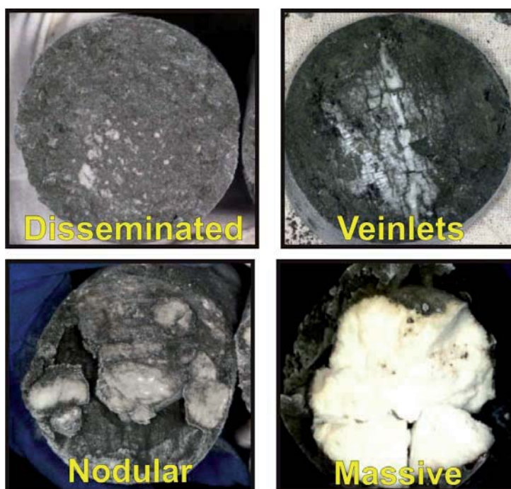
Figure 3.14. Gas hydrate fabrics identified onboard ODP Leg 204 at southern Hydrate Ridge, corresponding to the intervals: disseminated (ODP Leg 204-1249C-2H1, 108-140); veinlet (ODP Leg 204-1244C-8H1, 47-52); nodular (ODP Leg 204-1244C-10H2, 70-103); and massive (ODP Leg 204-1249C-1H-cc) (modified from Tréhu et al., 2003).
