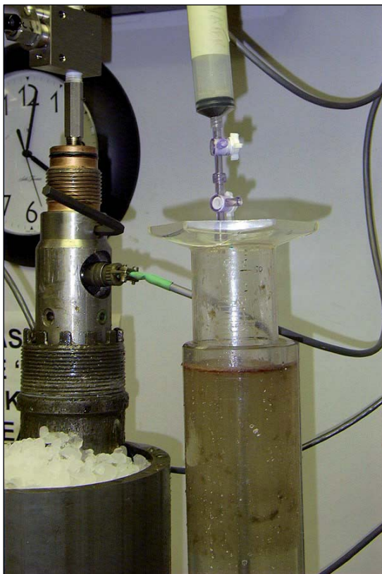
Figure 3.12. Pressure Core Sampler image showing the controlled release of gas in order to measure and analyse its in situ concentration.
