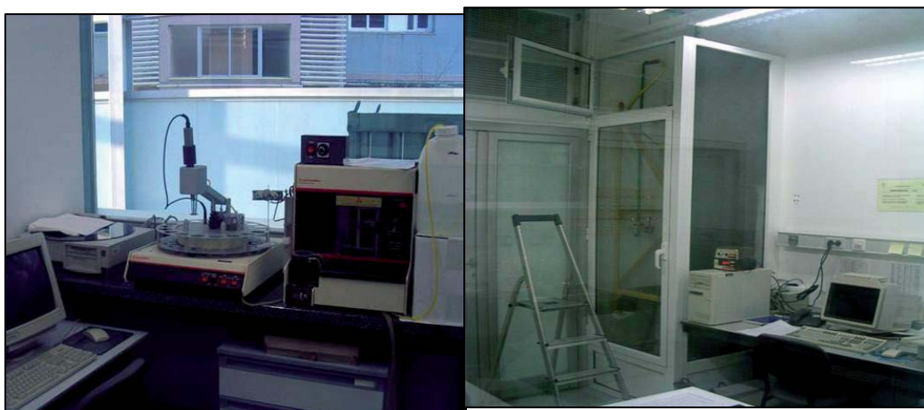
Figure 4.2. SediGraph and settling tube of the Institut de Ciències del Mar (CSIC) in Barcelona.
