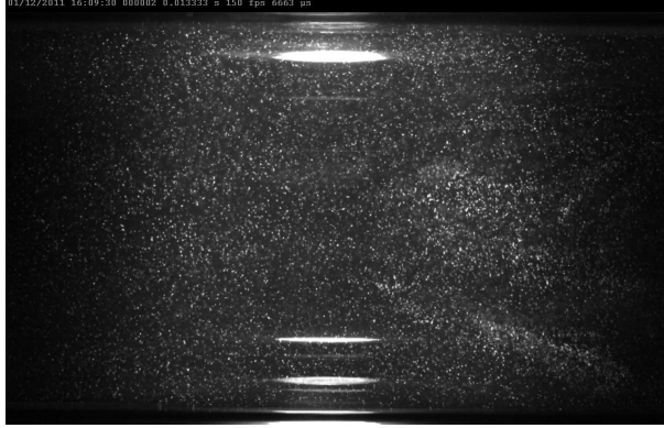
Figure 2.6: PIV image of a meridional plane of the tube (rotated by 90^\circ ). The seeding particles correspond to the bright dots. Small reflections are observed next to the tube walls.
