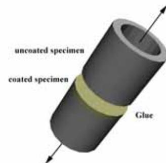
Figure 3.3. Set-up for the adherence test.
