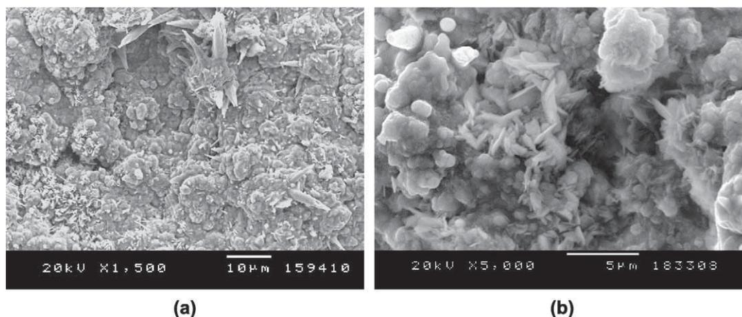
Fig. 7. Free surfaces of the as-deposited F2 coatings subjected to oxidation at 900 °C for 72 h showing (a) needles and whiskers and (b) cigar-like morphologies.
