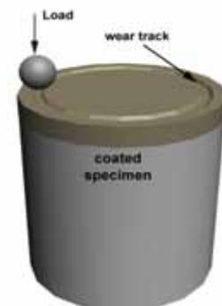
Figure 3.4. Set-up for the Ball-on disc test.
