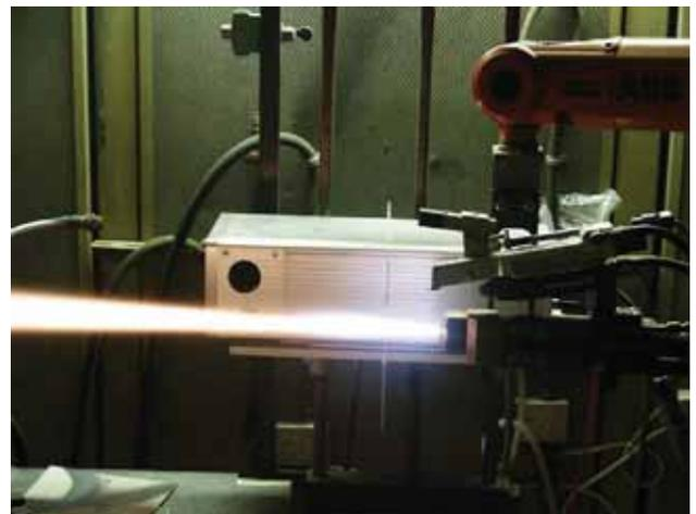
Fig. 1. Console and HVOF flame torch used in this work.
