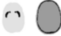
Figure 1. Activity and attenuation distributions in one section of the striatal phantom. Caudate and putamen basal ganglia can be observed in the activity image.
