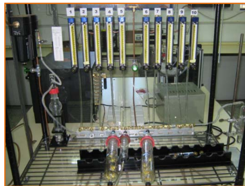
Fig. 4.2. Volatile collection of S. gregaria males by dynamic headspace extraction.
