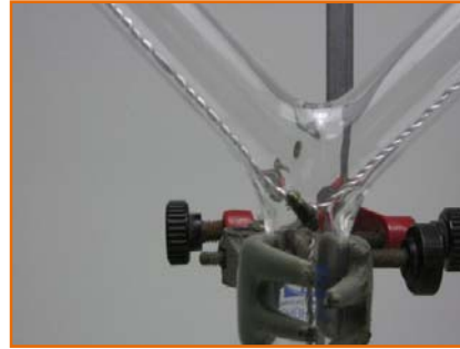
Fig. 14. Vertical posted Y-tube olfactometer used in laboratory bioassays to determine the attraction of C. florentinus adults to different odor sources (A) vs control (B).
