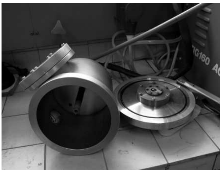
Figure 3.2: Detail of the inside of the arc-melting furnace chamber: cover with the cathode, on the left, and water-cooled Cu crucible (anode) with a sample above, on the right.
