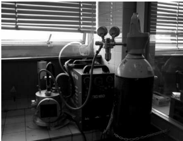
Figure 3.1: Complete view of the arc-melting furnace: chamber, power supply and Ar gas cylinder.
