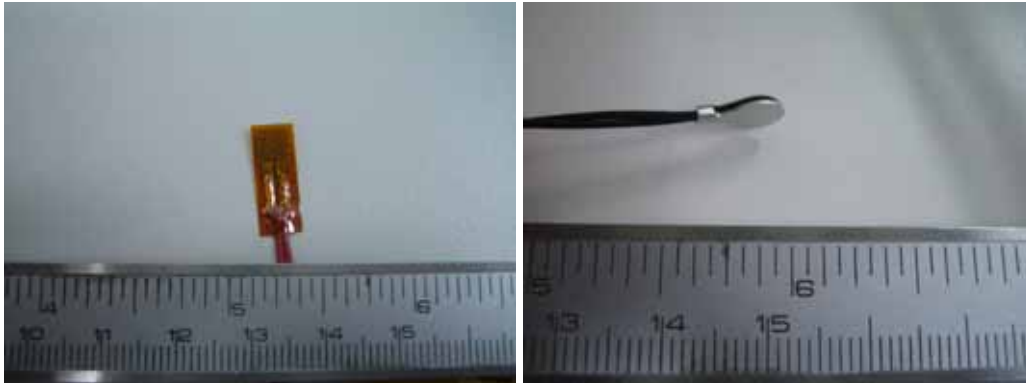
Figure 6.1: Left: 5.3 \Omega MINCO heaters. Right: Glass encapsulated Betatherm sensor
