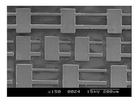
Figure 8. SEM image of released 10  $\mu m$  thick Co-11wt% Mo microstructures obtained on photolithographed silicon-based substrates.
