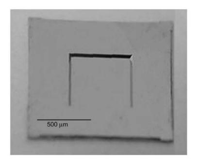
Figure 9. SEM image of a 7  $\mu m$  thick Co-40wt% Ni membrane with a silicon frame.
