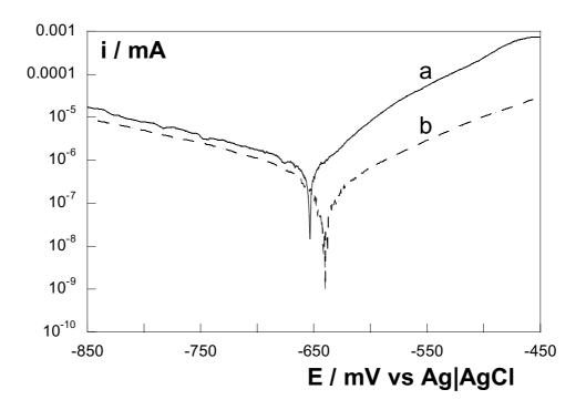
Figure 6. Potentiodynamic polarisation curves in 5% NaCl medium of 2  $\mu m$  thick (a) Co-11wt% Mo and (b) Co-12wt% Ni-13wt% Mo deposits.
