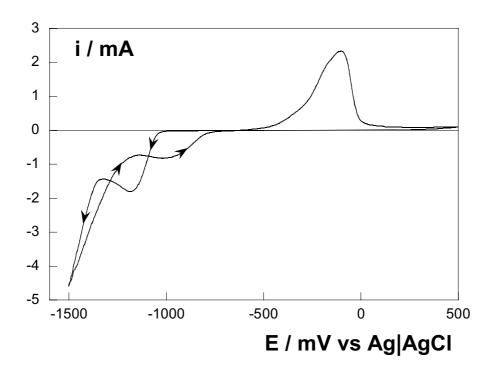
Figure 3. Cyclic voltammetry recorded at 50 mV  $\rm s^{-1}$  from a Co-Mo bath on vitreous carbon electrode (0.0314 cm<sup>2</sup>). Cathodic limit=-1500 mV, quiescent conditions.
