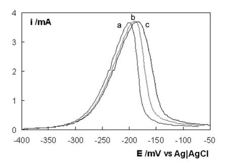
Figure 1. Stripping at 10 mV s<sup>-1</sup> of Co-Ni deposits obtained under the same deposition charge applying (a) -800, (b) -900 and (c) -1000 mV. Vitreous carbon electrode (0.0314 cm<sup>2</sup>), quiescent conditions.
