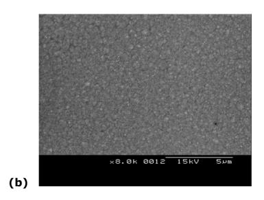
Figure 5. SEM images of (a) Co-11wt% Mo and (b) Co-12wt% Ni-13wt% Mo films.
