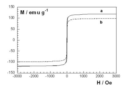
Figure 2. Hysteresis loops of 15  $\mu m$  thick Co-Ni deposits obtained at (a) -800 mV, 40 wt% Ni and (b) -950 mV, 53 wt% Ni.
