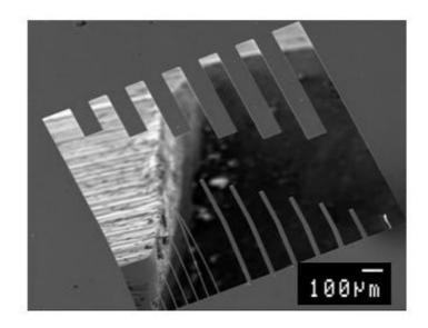
Figure 7. SEM image of a 7  $\mu m$  thick Co-40wt% Ni test microstructure.
