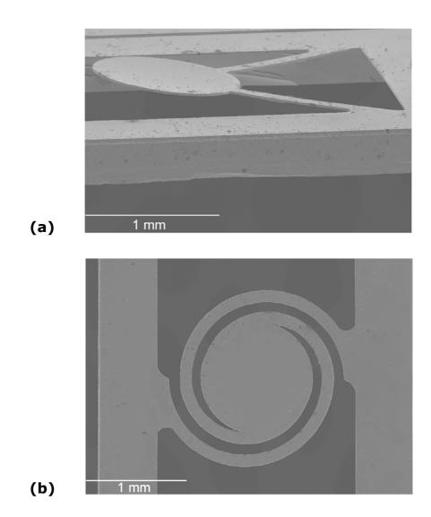
Figure 10. (a) and (b) SEM images of Co-12wt% Ni-13wt% Mo micromachined pieces.
