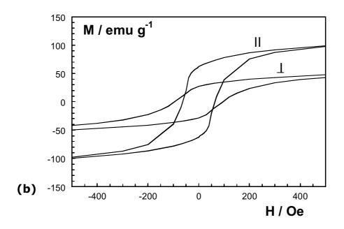
Figure 4. (a) Parallel and perpendicular hysteresis loops and (b) magnified detail of a 2  $\mu m$  thick Co-11 wt% Mo deposit.
