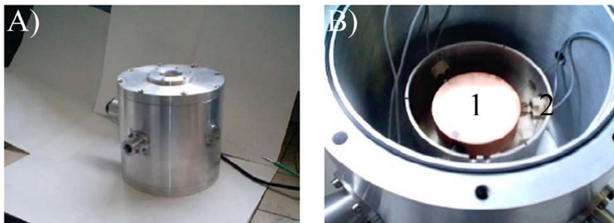
Figure 3.6. A) Oven employed to perform the thermal treatments. B) View of the copper block (1) and the heating system (2).
