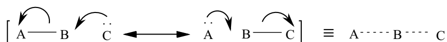
Figure 5. Lewis structure of a 3c-4e bond model, which is represented by two resonance structures.
