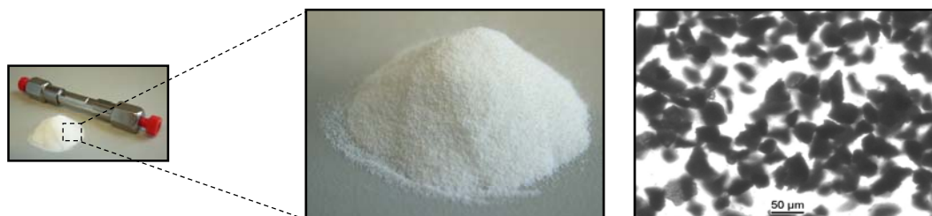
Figure 2.10: Molecular imprinted polymer after being milled and sieved. On the right a picture obtained with an optical microscope of the homogeneous particle material.
