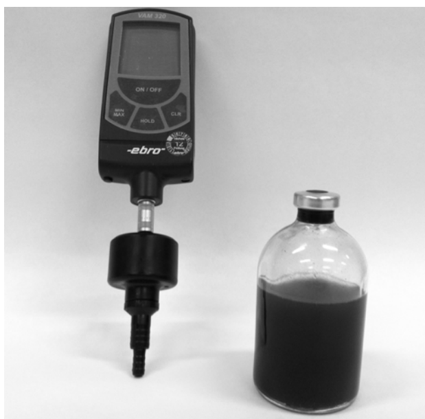
Fig. 3.1. BMP serum bottles and vacuumeter used in this study
