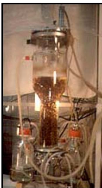
Figure 5. Configuration of a 5 L air-lift bioreactor used to culture T. baccata immobilized cells.
