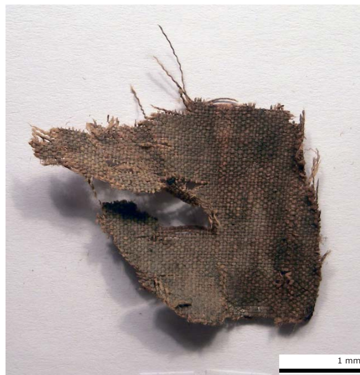
Figure 3. Example of a very degraded sample with an acidic pH of 4.8 and a low DP of 410. The threads of this sample could be easily broken just by pulling them with the fingers.
