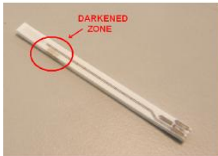
Fig. 5. Darkened aspect of the solid ceramic of one of the sensors after applying the external polarization.
