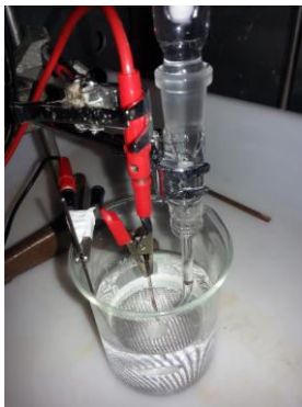
Figure 2 – Experimental setup for corrosion measurements (left: counter-electrode; middle: sample; right: reference electrode).
