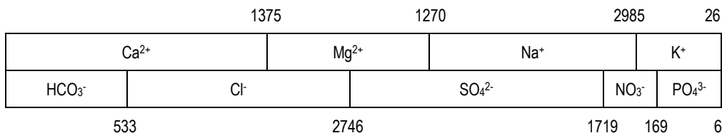
Figure 8.12 Bar diagram of feed water from Goodyear in mg/L as \text{CaCO}_3 (Self production)
