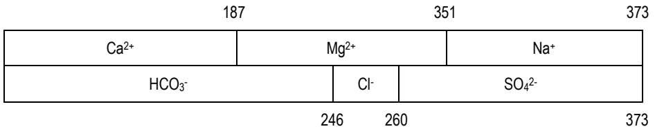
Figure 3.1 Bar diagram of raw water in mg/L as \text{CaCO}_3 (Self production from [4])
