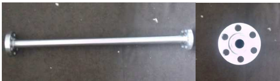
Figure 17. Stainless steel tubular reactor. Frontal and lateral view.
