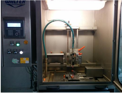
Figure 5.8. Testing machine with pressurized water
