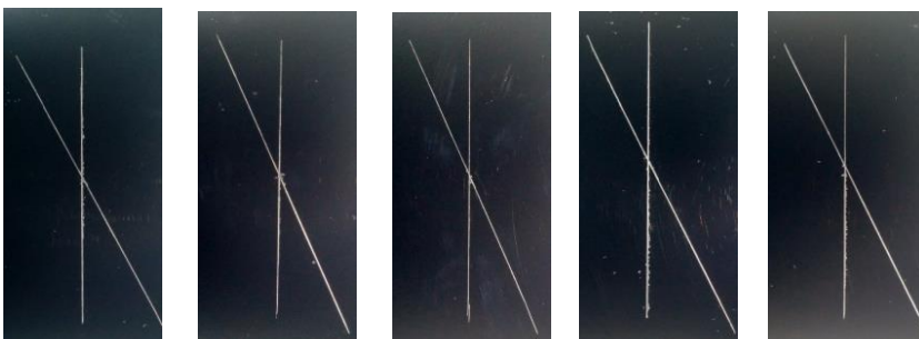
Figure 6.4. Pressurized water test according the standard of Volkswagen with prototypes A (left), B, C, D and E (right) applied with hardener 2
