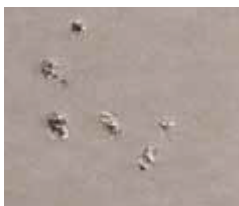
Figure 3.6. Paint defect. Inclusions. ( Image from Paints defects, reference 4 )
