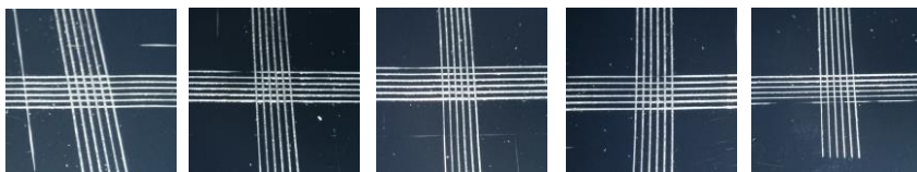
Figure 6.2. Adherence of prototypes A (left), B, C, D and E (right) applied with the hardener 2
