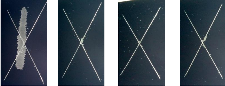
Figure 6.18. Pressurized water test according the standard of PSA with prototypes H (left), I, J and K (right) applied with hardener 2
