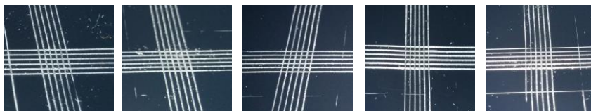
Figure 6.1. Adherence of prototypes A (left), B, C, D and E (right) applied with the hardener 1
