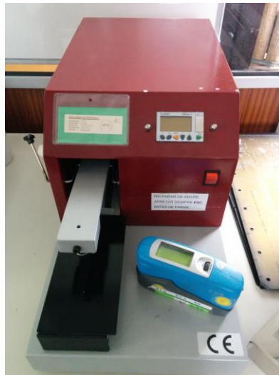
Figure 5.10. Crockmeter used by the abrasion test Ford and micro-gloss BYK Gardner
