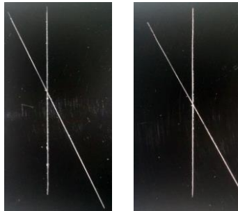
Figure 6.12. Pressurized water test according the standard of Volkswagen with prototypes F (left) and G (right) applied with hardener 1
