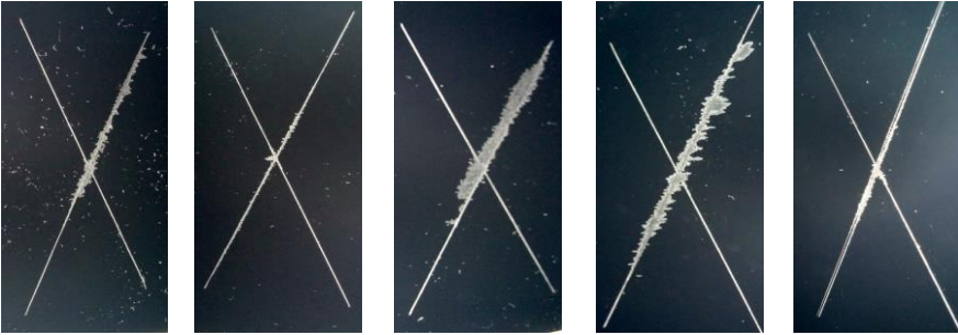
Figure 6.5. Pressurized water test according the standard of PSA with prototypes A (left), B, C, D and E (right) applied with hardener 1
