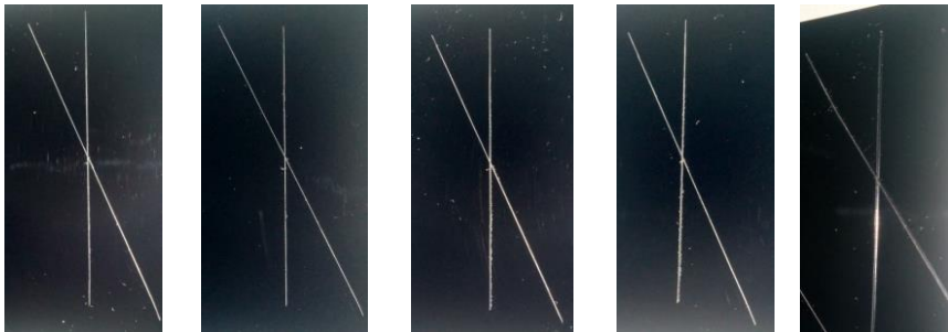
Figure 6.3. Pressurized water test according the standard of Volkswagen with prototypes A (left), B, C, D and E (right) applied with hardener 1
