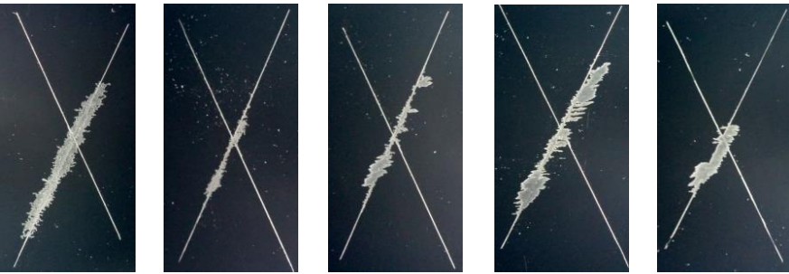
Figure 6.6. Pressurized water test according the standard of PSA with prototypes A (left), B, C, D and E (right) applied with hardener 2
