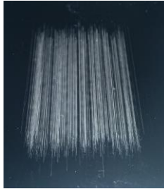
Figure 6.8. Example of Renault scratch. Prototype C using hardener 1
