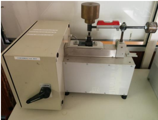
Figure 5.9. Crockmeter used for Renault abrasion test.
