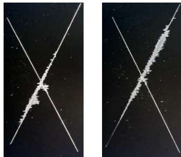
Figure 6.14. Pressurized water test according the standard of PSA with prototypes F (left) and G (right) applied with hardener 1
