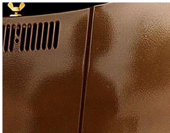
Figure 3.5. Paint defect. Orange peel. (Image from Paints defects , reference 4)
