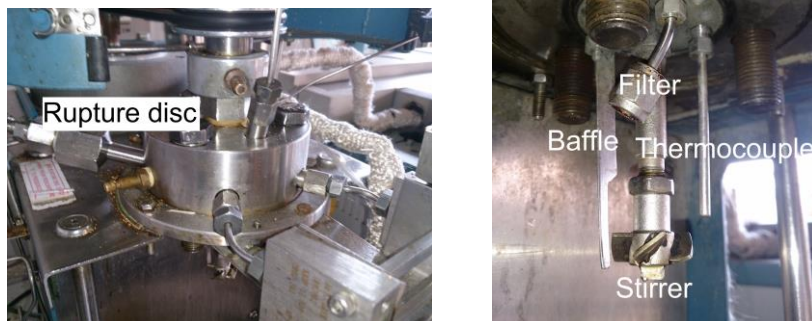
Figure 8 and 9. Tank head with internal accessories.
