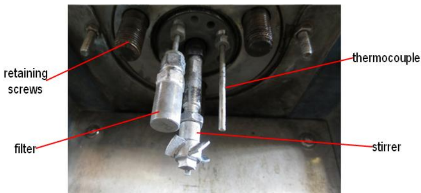
Fig 6.A look into the internal accessories of the reactor.
