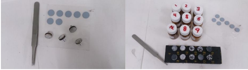
Figure 9. Left: Material for preparation SEM. Right: sample holder with the mesoporous material.
