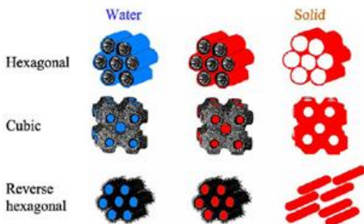
Figure2. It shows a surfactant liquid crystal first solidified and then transformed into a mesoporous material by removal of the surfactant. Surfactant removal can be made either by washing or by calcinations [24].
