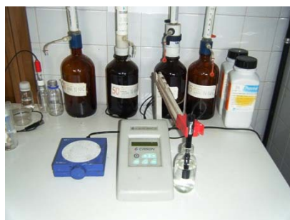
Figure 3.7. Ammonia electrode (pH/mV Crison MicropH 2002)
