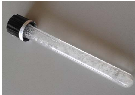
Figure 3.13. PHA extracted from biomass
