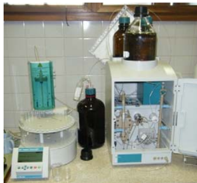
Figure 3.8. Ionic chromatograph (Metrohm Advanced Compact IC)
