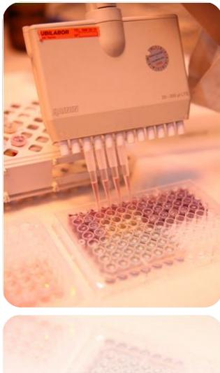
The colorimetric reaction takes place in 96-well plates.
