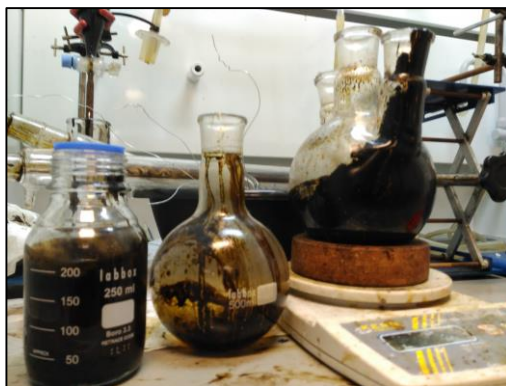
Figure 10: Detail of the condensation system (a) and the two tanks (the two balloons) after the pyrolysis test.
