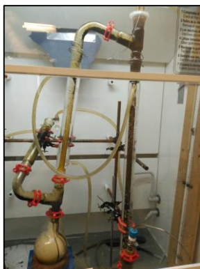
Figure 10: Detail of the condensation system (a) and the two tanks (the two balloons) after the pyrolysis test.
