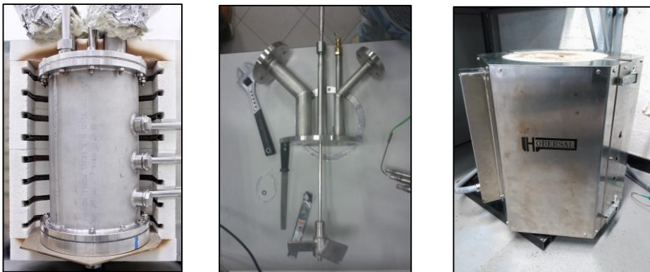
Figure 4: Detail of the reactor (a), the agitator and top orifices (b), and the closed oven (c).
