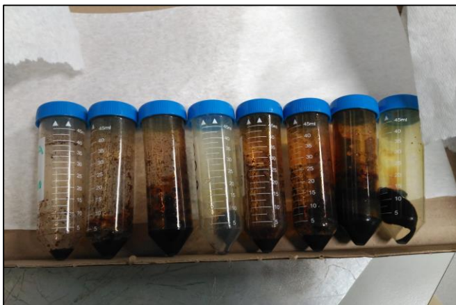
Figure 15: Detail of the eight samples of oil mixed with water after the first extraction.
