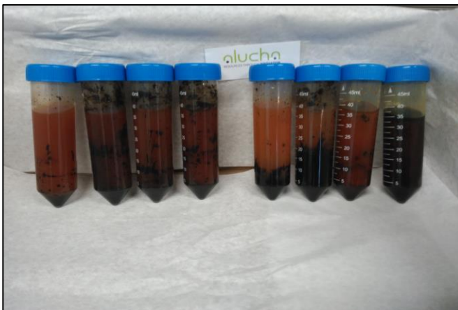
Figure 14: Detail of the eight samples of oil mixed with water before the first extraction.
