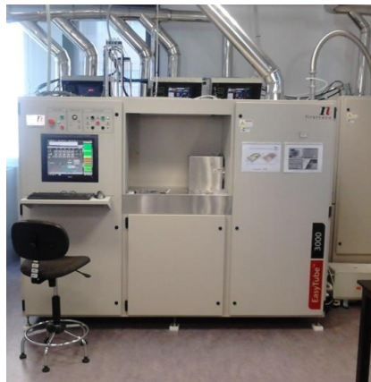
Figure 2.9: Nano EasyTube® 3000 equipment used in this work for depositing polysilicon films (located at IREC)
