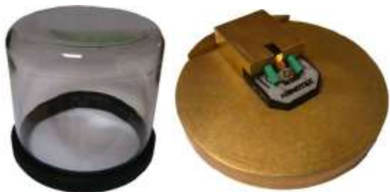
Image 3.7 AFM head glass cover and cantilever exchange bay.
