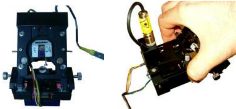
Image 3.8 (Left) Cantilever holder in the head.(Right) Handling the AFM head.
