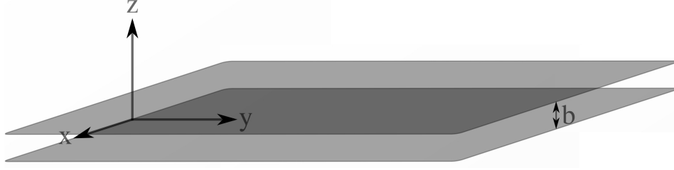
Figure 4: Scheme of a Hele Shaw geometry. The front of fluid advances between two infinite plates separated a small distance b
