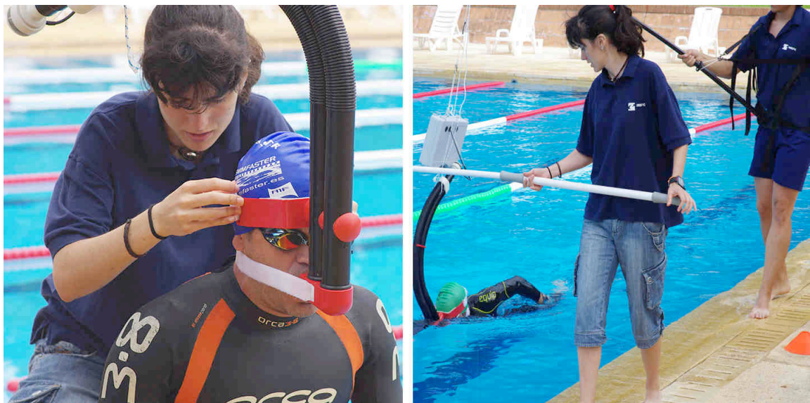
Figure 6. Subjects performing the swimming test with the respiratory snorkel and valve system for breath-by-breath gas analysis.
