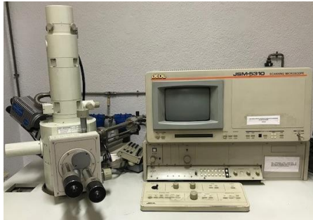
Figure 9: Scanning electron microscope equipment used.
