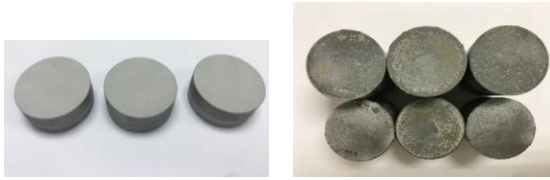
Figure 26: Bilayer coating before (left) and after (right) tensile strength test.
