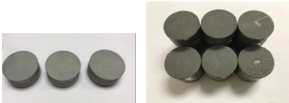
Figure 28: Graded coating before (left) and after (right) tensile strength test.
