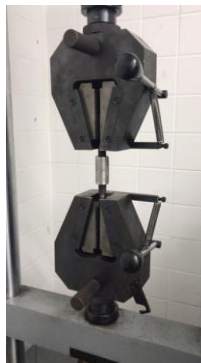
Figure 13: Equipment used to evaluate coatings tensile strength.
