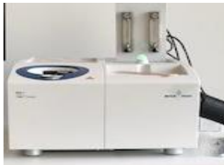
Figure 10: Differential Scanning Calorimetry (DSC) equipment used.
