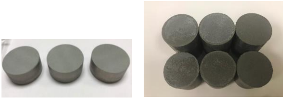
Figure 27: Blended coating before (left) and after (right) tensile strength test.
