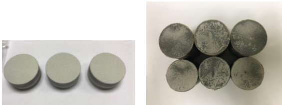
Figure 29: Agglomerates coating before (left) and after (right) tensile strength test.
