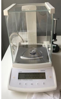
Figure 15: Laboratory balance used to weight each sample of this study.
