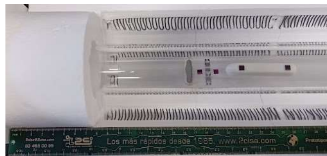
FIG. 2: Distribution of precursor and samples along the furnace.
