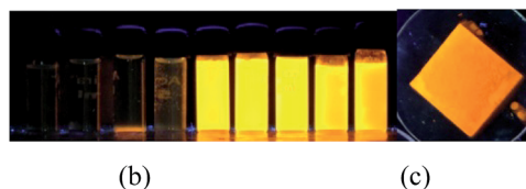
Fig. 4 (a) PL spectra of 1 in MeOH/water mixed solvents with different f_w (water fraction). Inset: variation of the PL intensity with respect to water contents. (b) Luminescent images of 1 in solutions with different water fractions (c) image for a solid sample of 1 under irradiation with a 365 nm UV lamp [ c = 10 \times 10^{-5} M].
