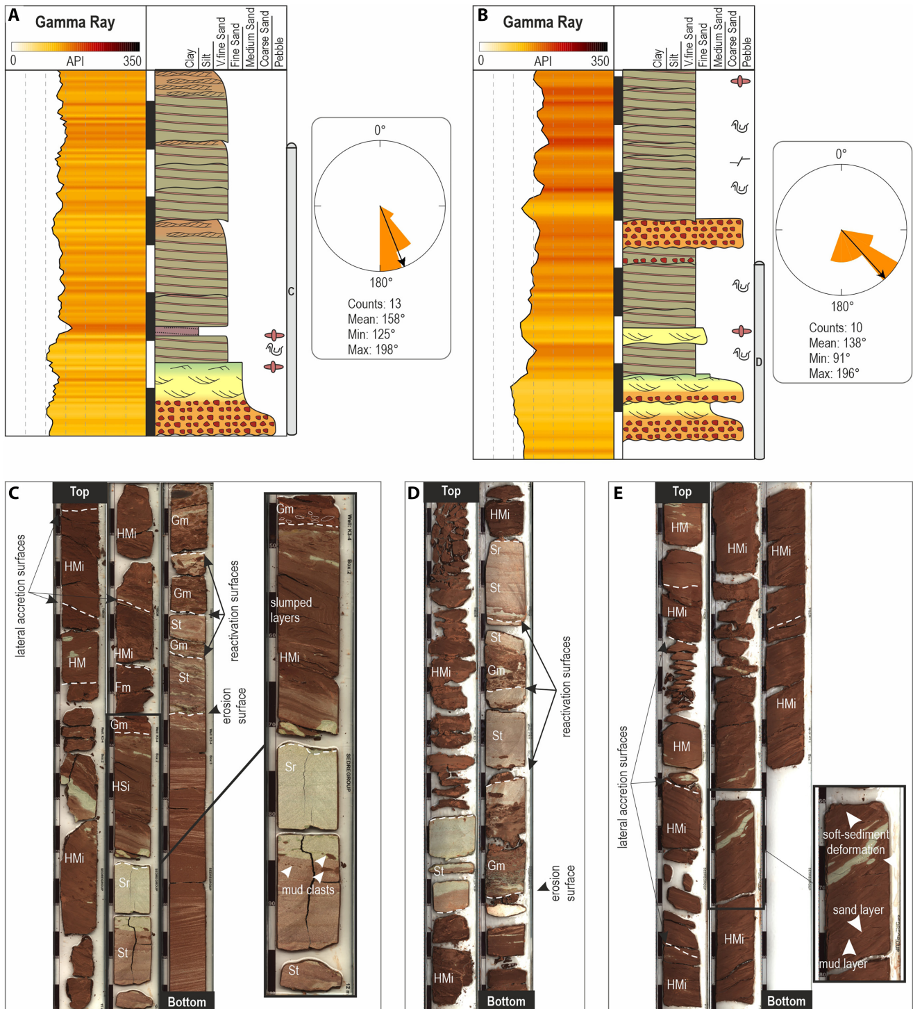
FIGURE 12 Subsurface data from the tide-dominated point bar example (Point bar geobody 3). (A) Gamma ray log, sedimentological log and azimuth rose diagram of lateral accretion surfaces from Well K3-4. (B) Gamma ray log, sedimentological log and palaeocurrent rose diagram from Well K3-2. (C-E) Slabbed core views from Wells K3-4, K3-2 and K3-1, respectively. See Figure 9 for the locations of the wells.
