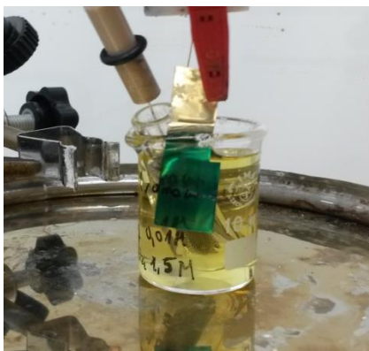
Figura 22. Adsorption of reduced MBQ on Pt surface.
