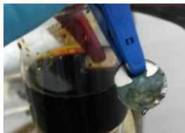
Figura 29. Adsorption of reduced MBQ on Ni surface
