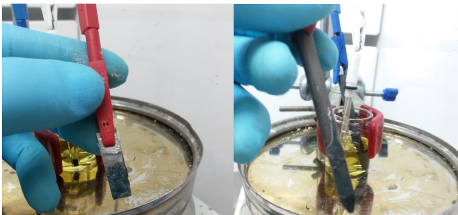
Figura 24. Adsorption of reduced MBQ on flexible graphite (left), and graphite rod (right)
